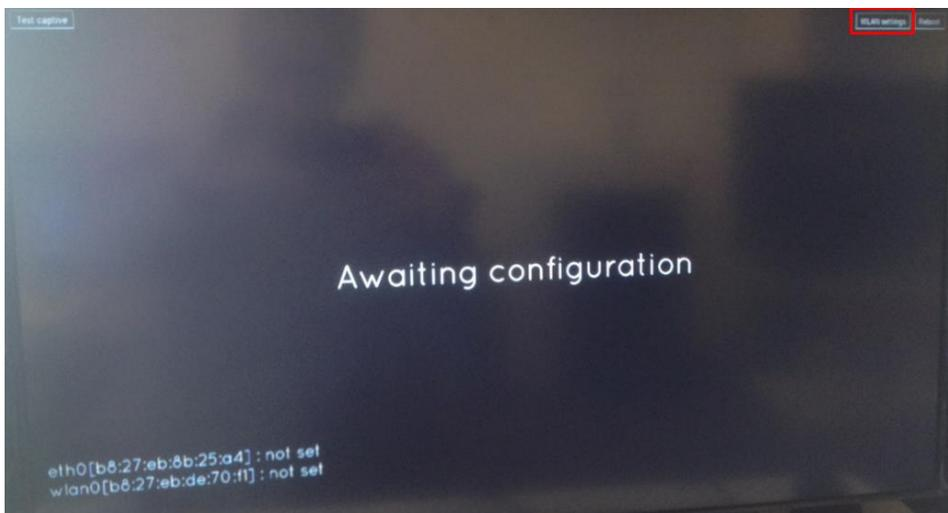
6. Connect a USB mouse to the Raspberry PI and select the "WLAN settings" button.
